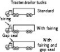
Tractor-trailer trucks | Standard<br>With fairing<br>With fairing and gap seal | Frontal area<br>Frontal area<br>Frontal area                                                                                                                                                                                                                                                                             |          |       |     |      |               |      |      |      |              |      |      |      |
